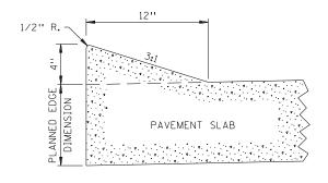
CUBIC YARDS OF CONCRETE PER LINEAL FOOT = 0.0062 LINEAL FEET PER CUBIC YARD OF CONCRETE = 162.0
